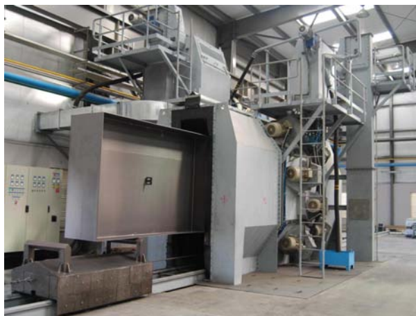
12 Wheel Shot Blasting Machine for 2m high x 0.8m wide Product
